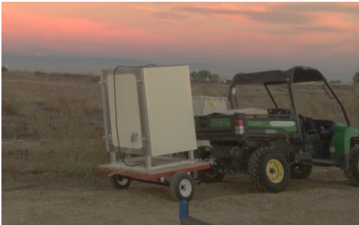
Figure 3-2. Transportable Ambient Air Quality Analyzer Calibration System
