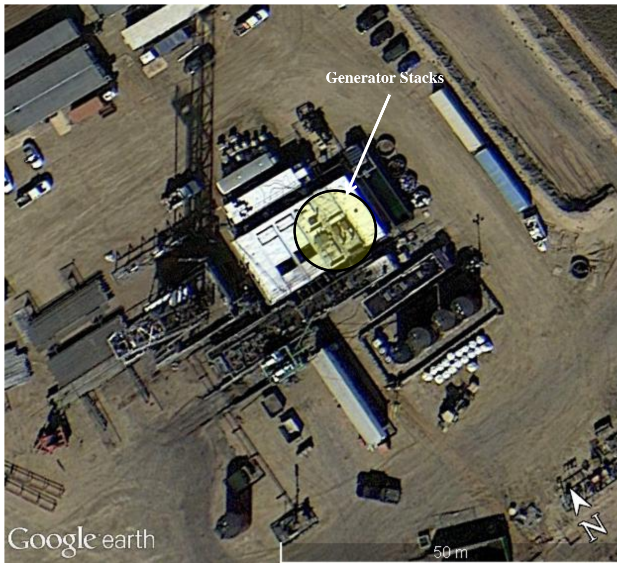
Figure 2-6. Aerial Photograph Looking Down at the Generator Trailers and Other Drill Rig Structures
