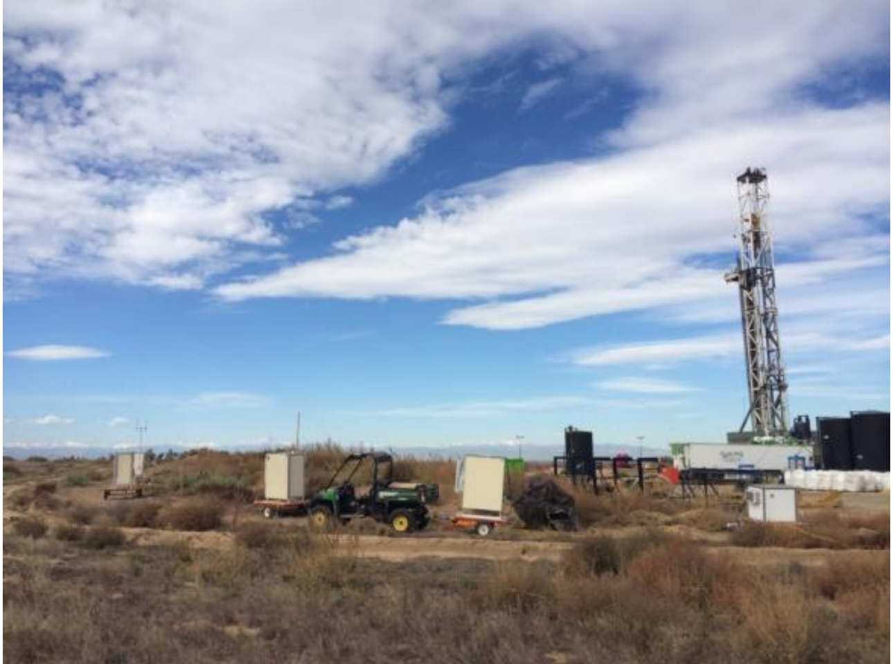
Figure 4-6. Monitoring Sites 9 through 12 Wrapping Around the Southeast Corner of the Well Pad (West of Site 12, the dune to the right obstructs wind flow to sites along the perimeter easement)
